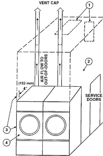
**DRYER INSTALLATION WITH SEPARATE EXHAUST (PREFERRED)**
