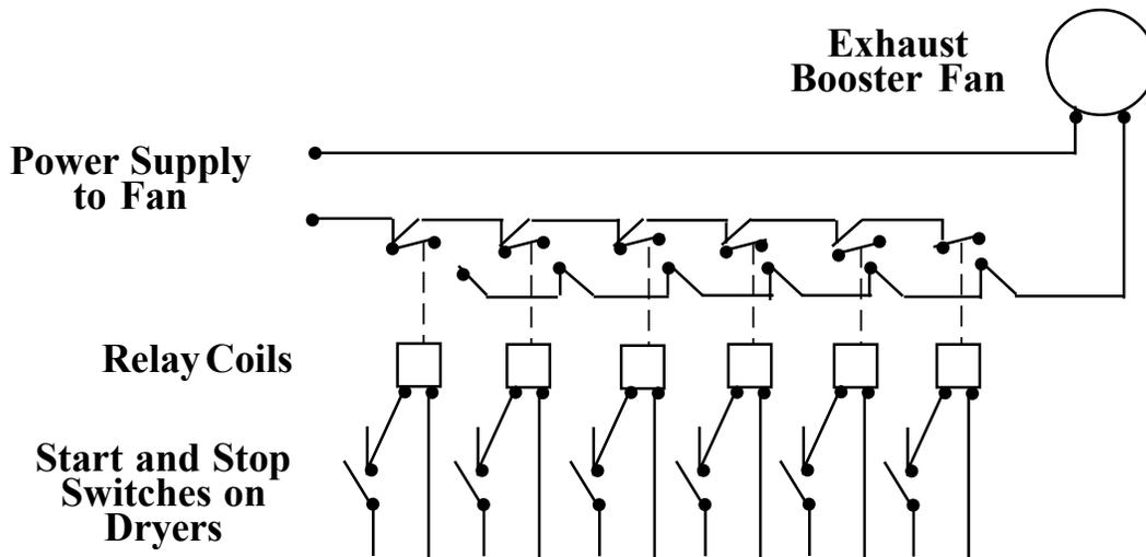
*Dryer Installation with Multiple Exhaust (Illustration)*
